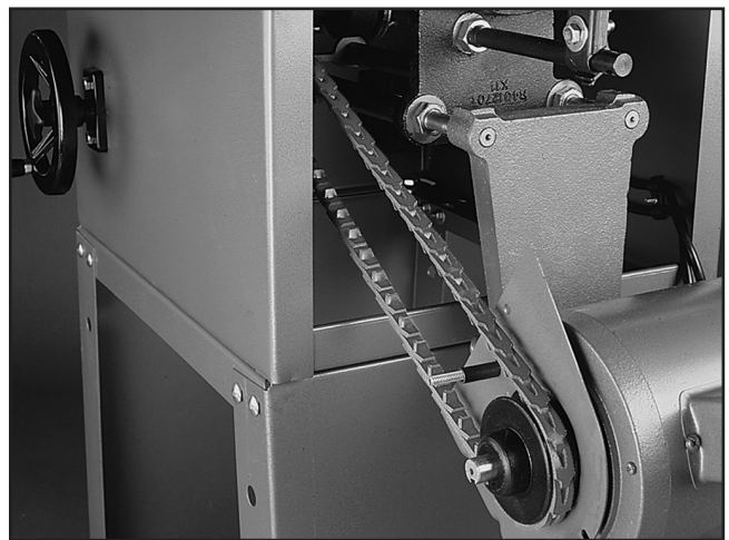
Figure 37. G3640 Power Twist® V-Belt installed.
